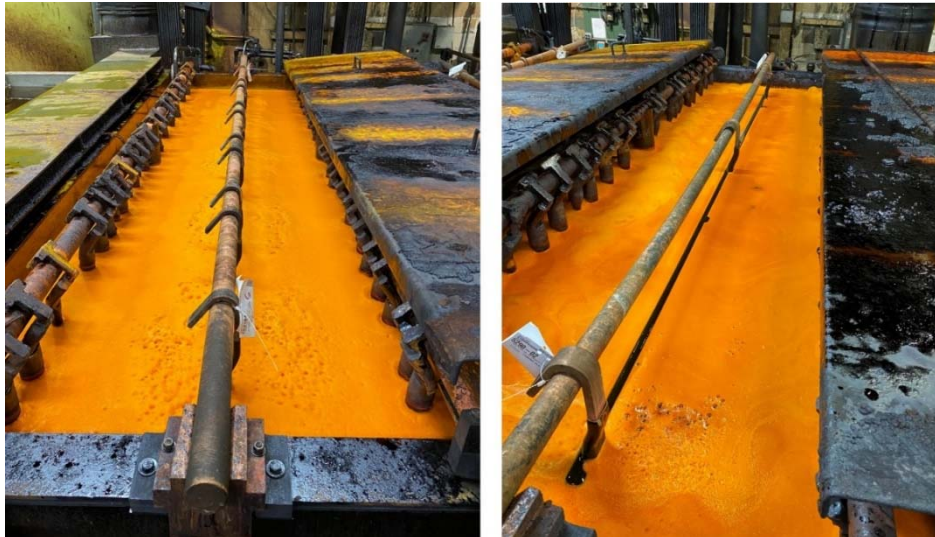
Figure 3 – Comparison of Non-PFAS baths: (L) New makeup versus (R) Slide conversion after two weeks of operation.
