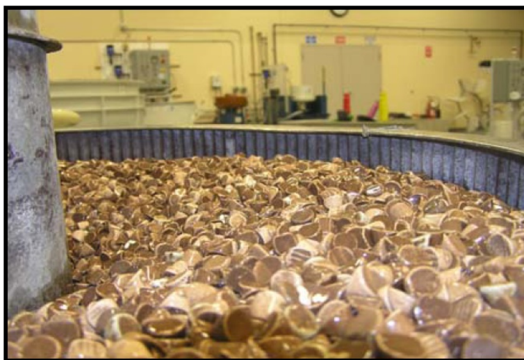
Figure 2 - Image of a vibratory bowl with the proper depth of media present in the bowl channel. 6
